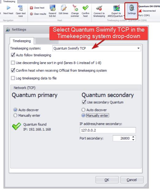
In the timekeeping settings window you must select Timekeeping system: Quantum Swimify TCP. You will then get a group box named Network (TCP) at the bottom of the settings window with some additional settings that are specific for Quantum Swimify TCP.
