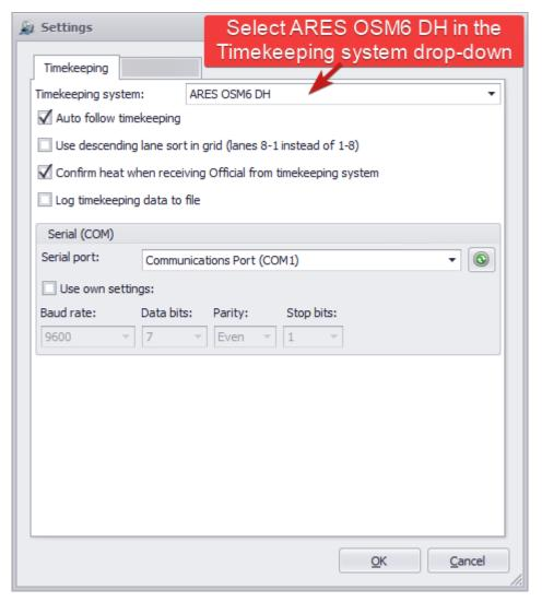
In the timekeeping settings window you must select Timekeeping system: ARES OSM6 DH. You will then get a group box named Serial (COM) at the bottom of the settings window with some additional settings that are important that you set correctly. You must select the correct Serial Port in the drop-down box.
