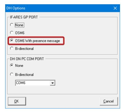
Click OK button to close the DH Options window and then open the menu named DH and make sure that the menu selection On is enabled and has a checkmark.
