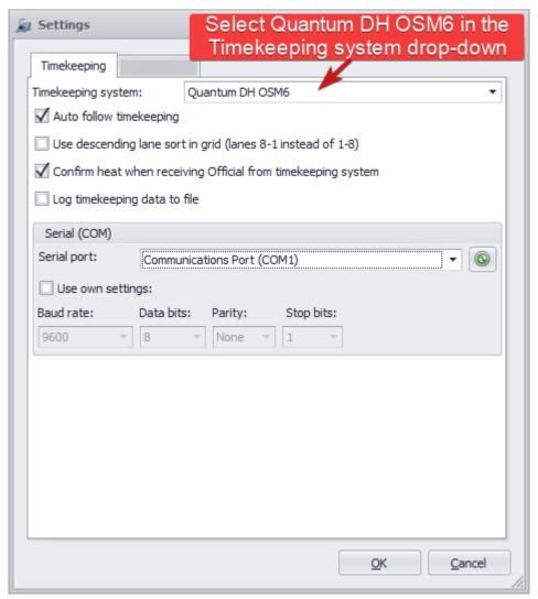
In the timekeeping settings window you must select Timekeeping system: Quantum DH OSM6. You will then get a group box named Serial (COM) at the bottom of the settings window with some additional settings that are important that you set correctly. You must select the correct Serial Port in the drop-down box.
