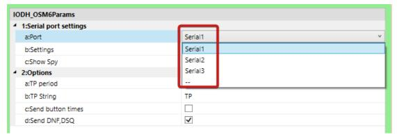
The different options that you can select in this drop-down box (Serial1, Serial2 etc) corresponds to the physical outputs on the Quantum unit that is marked Serial 1, Serial 2 etc. So if you connect the cable to the output named Serial 1 then you must select Serial1 in the drop-down box.
