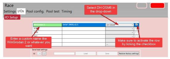
Before you can activate the row by clicking in the checkbox you must first select which serial port you are using on the Quantum unit for this protocol. You change this setting in the bottom grid on the row that says "a:Port", see image below.
